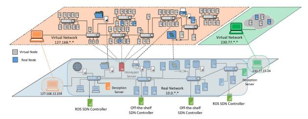
Fig. 6. Emulated enterprise test network.
