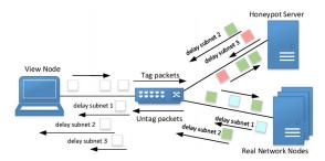
Fig. 5. Tagging packets to add artificial delay.
